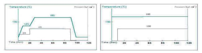
传压参数根据不同设备及产品规格需作相应调整;采用快压方式,后固化条件是 160-180℃、60-90 分钟。 The parameters of hot Pressure need to be adjusted according to different equipment and product specifications. After fast press, the curing condition is 160-180℃ for 60-90min.
